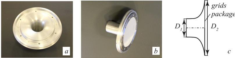
FIG. 6. Short diffuser without (a) and with the metal grid package at the outlet (b) and the scheme of short diffuser (c).
