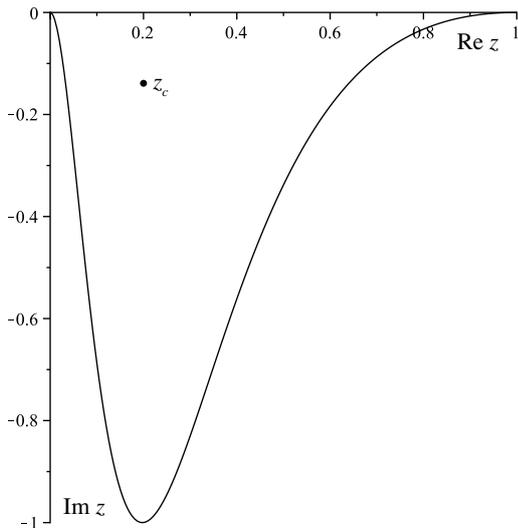
Figure 2: Integration path chosen for solving the Rayleigh equation for the velocity profile  $u_0(\eta) = M_\infty \sin(\pi\eta/2)$ ,  $M_\infty = 1.6$ ,  $c = 0.5 - 0.33i$ . The critical point is  $z_c \approx 0.20 - 0.14i$ .
